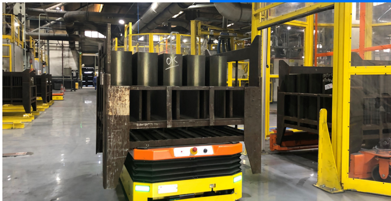
Use of autonomous vehicles for internal transportation of parts at Fras-le reduces risks for professionals
